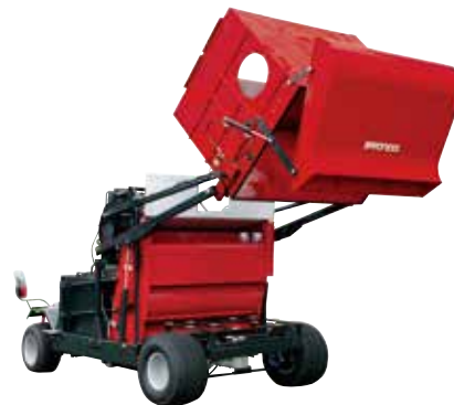
Grass-catching bucket can be raised 68.9in (175cm) from ground.
